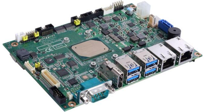
The low power embedded board provides rich I/O including two USB 2.0 and four USB 3.0; there are two LAN ports and four COM ports, with two RS-232/422/485 and two RS-232. The display interface consists of one HDMI and one LVDS, while VGA and eDP are optional. In addition, it features two PCI Express Mini Card slots for various peripheral modules such as Wi-Fi, 3G, and 4G LTE.
