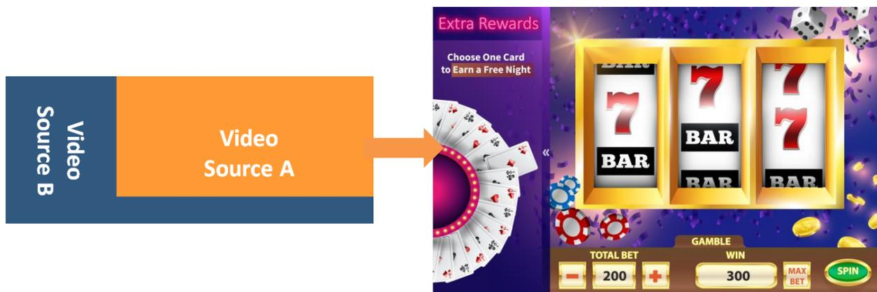
(Illustration of how a game display in picture-in-picture mode is split up into two areas showing the contents of two different video sources.)
