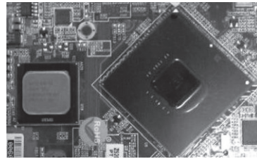
Intel® Z520PT with US15WPT supports wide temperature of -40°C ~ +70°C
