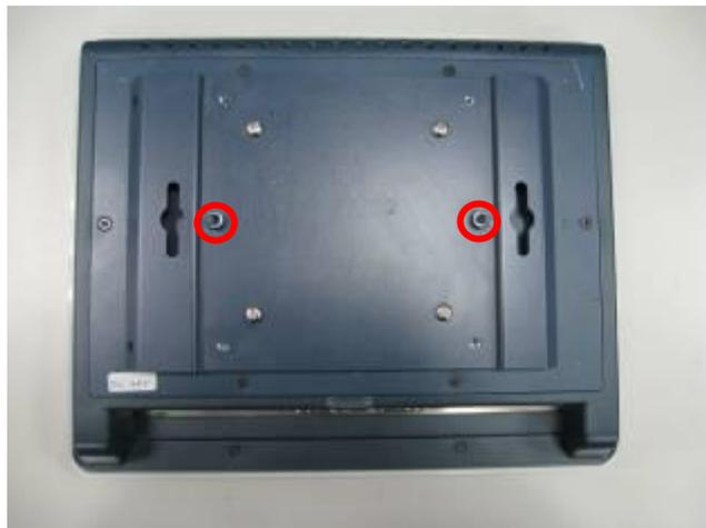
**Step 2 Assemble the desktop stand to the chassis, and fix the screws.**
