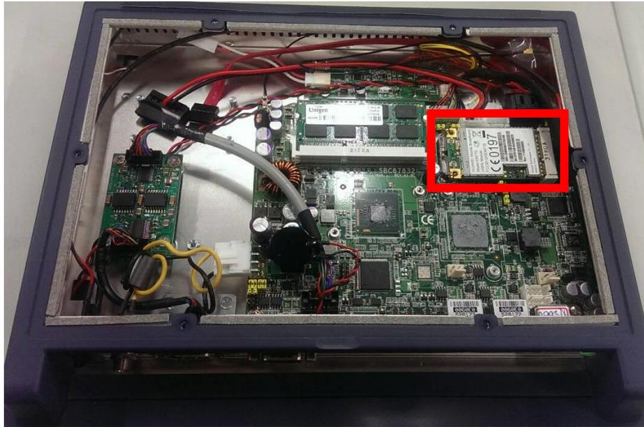
**Step 2** The socket latches are clipped on to the edges of the Mini card. Install wireless LAN card to the socket.
