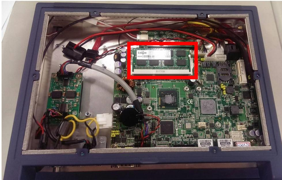
**Step 2** Insert the DRAM to the DIMM socket, and then push it down firmly until it is clipped by the socket.
