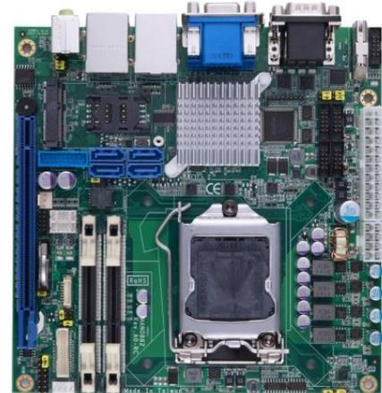
The industrial-grade MANO882 provides rich I/O connections including six COM ports (two RS-232/422/485 and four RS-232), four SATA-600 with RAID 0/1/5/10 function, dual Gigabit LAN ports, six USB 2.0 ports, four USB 3.0 ports, and eight channels digital I/O (4-IN and 4-OUT). Additionally, the MANO882 supports hardware monitoring and watchdog timer. It also offers long term support and reliable quality.
