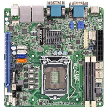
Axiomtek's MANO881 comes with advanced connectivity including three RS-232-232/422/485 ports, three RS-232 ports, two USB 3.0 ports, eight USB 2.0 ports, two SATA-600, two SATA-300, two Gigabit LANs, HDMI, LVDS, VGA, digital I/O (8 channel programmable), and HD audio. Expansion capabilities include one PCIe x16 slot and mSATA socket. The motherboard supports watchdog timer and SMART FAN. The MANO881 also meets all requirements for the Windows® 7 and 8 OS.
